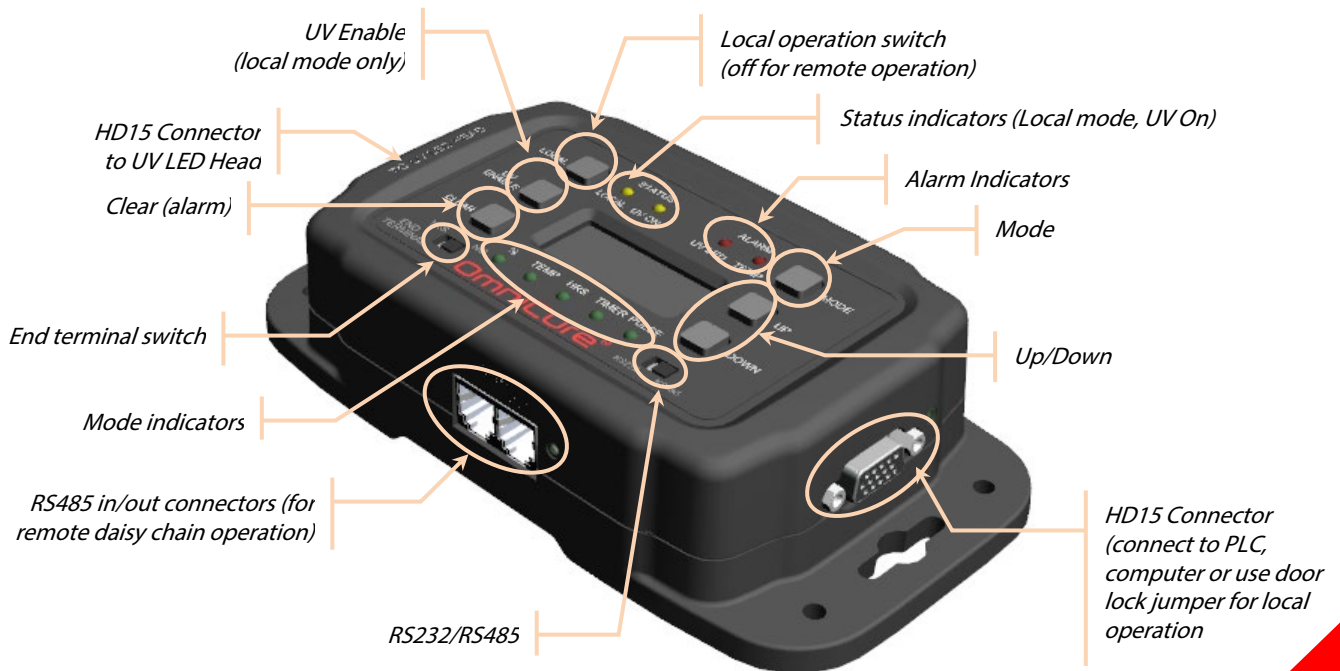
Figure 4 PLC2000 Remote Control Console
